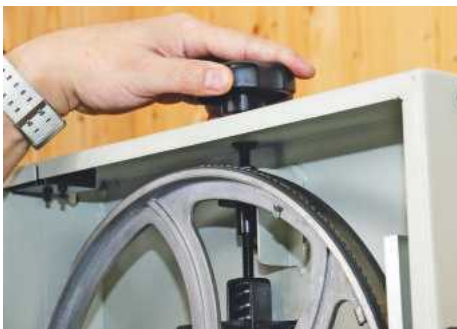
▲ Initial tensioning is achieved with the top adjuster
